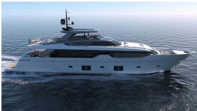
She will be Sanlorenzo's first asymmetrical yacht, featuring a unique single side deck on the starboard side. The layout allows the main deck interior to expand outboard to the hull and superstructure limits. The boat's asymmetric design has its genesis in the partnership Sanlorenzo announced in 2015 with American car designer and BMW guru of many years Chris Bangle, but its development was entrusted to Zuccon International Studio.
