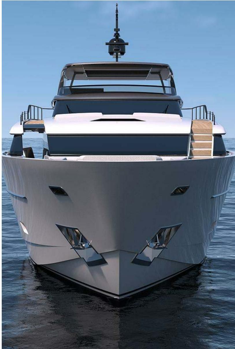
The SL102 otherwise will be a typical planing hull, with top speed expected to be around 28-29 knots, depending on the selection of engines (twin 16V MTU M86 or the upgrade M96). Cruising speed will be around 25-26 knots, and the yacht will be able to carry 12,000 litres of fuel and 2,000 litres of water.
