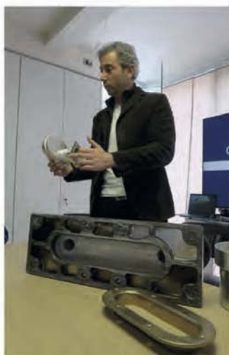
▲ Custom specialists Rossinavi design and manufacture many of their components for their unique builds, such as this bollard. Note the sculpting of the underside to reduce weight
