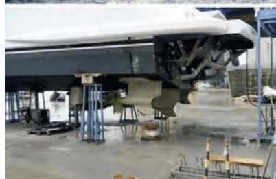
▲ Multiple IPS drives, in threes and fours, are becoming more common due to easier installation and improved performance
