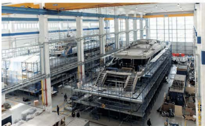
▲ Companies that have traditionally moulded in GRP, such as Overmarine (Mangusta), have moved to aluminium as their craft have become bigger. Here a pair of Mangusta 54m Grand Sport yachts are under construction at its modern facility near Pisa
