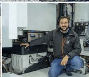
▲ Volvo Penta's Stefano Pesci in the engine room of the Amer 110. To his right is one of the four IPS 1050 installations
