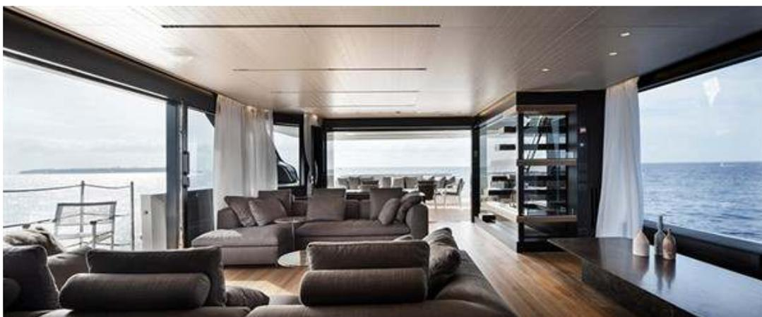
Aiming to obtain greater usability of the interior spaces and better access to the exterior, the SL102 recovers about 10sqm of area for the interior by only keeping the deck on starboard. This allows a large dining room with full-height window that overlooks the sea, while on the other side to starboard, a living room opens on a balcony.
