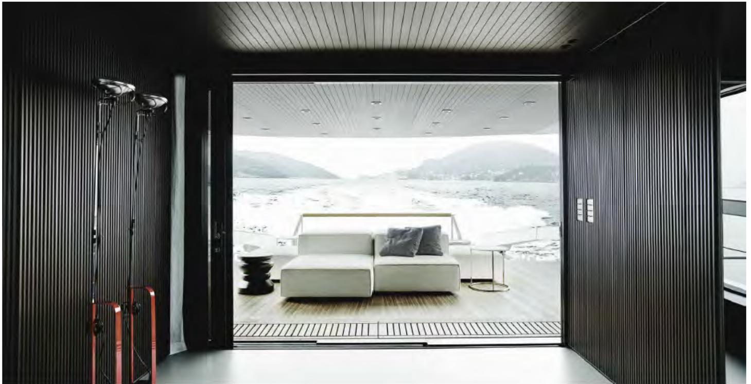
A key feature of the SX88 is the open stern. Naval architect Ivan Santella wanted guests to be closer to the sea, so they step down from the aft deck to a large beach club with a glass-banking platform that can be lowered into the water.
